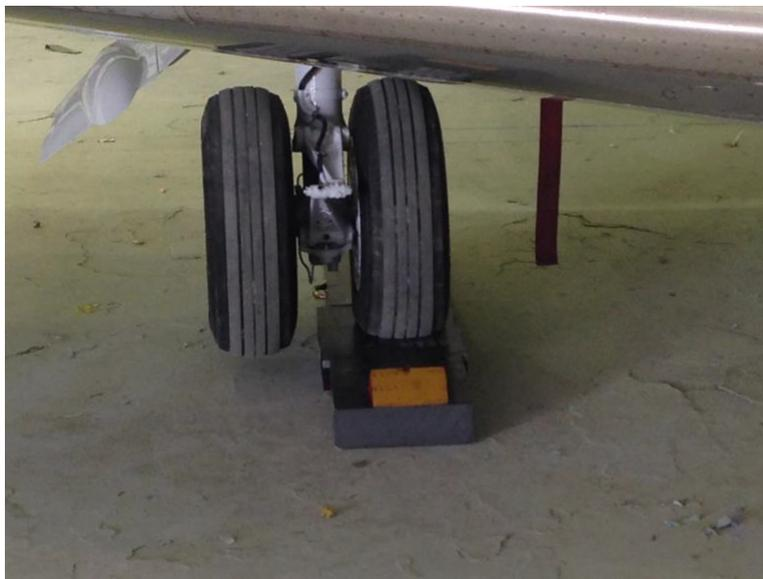
**Always check to make sure the wheel off the platform is not touching the floor.**
