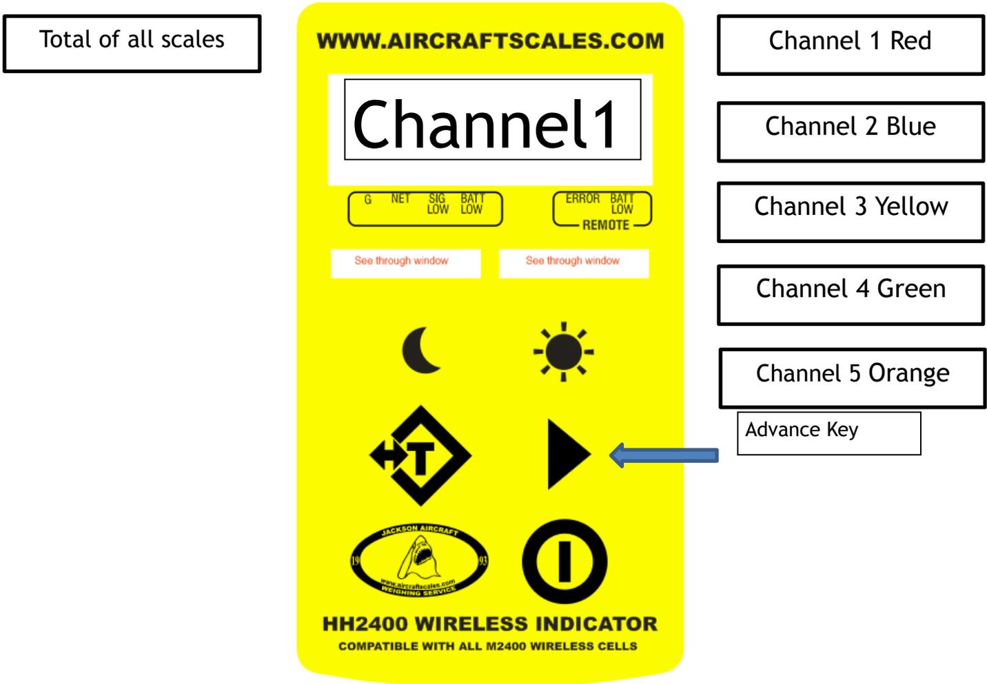
Pressing the advance key while reading “Channel 1” will move the indicator to “Channel 2”
