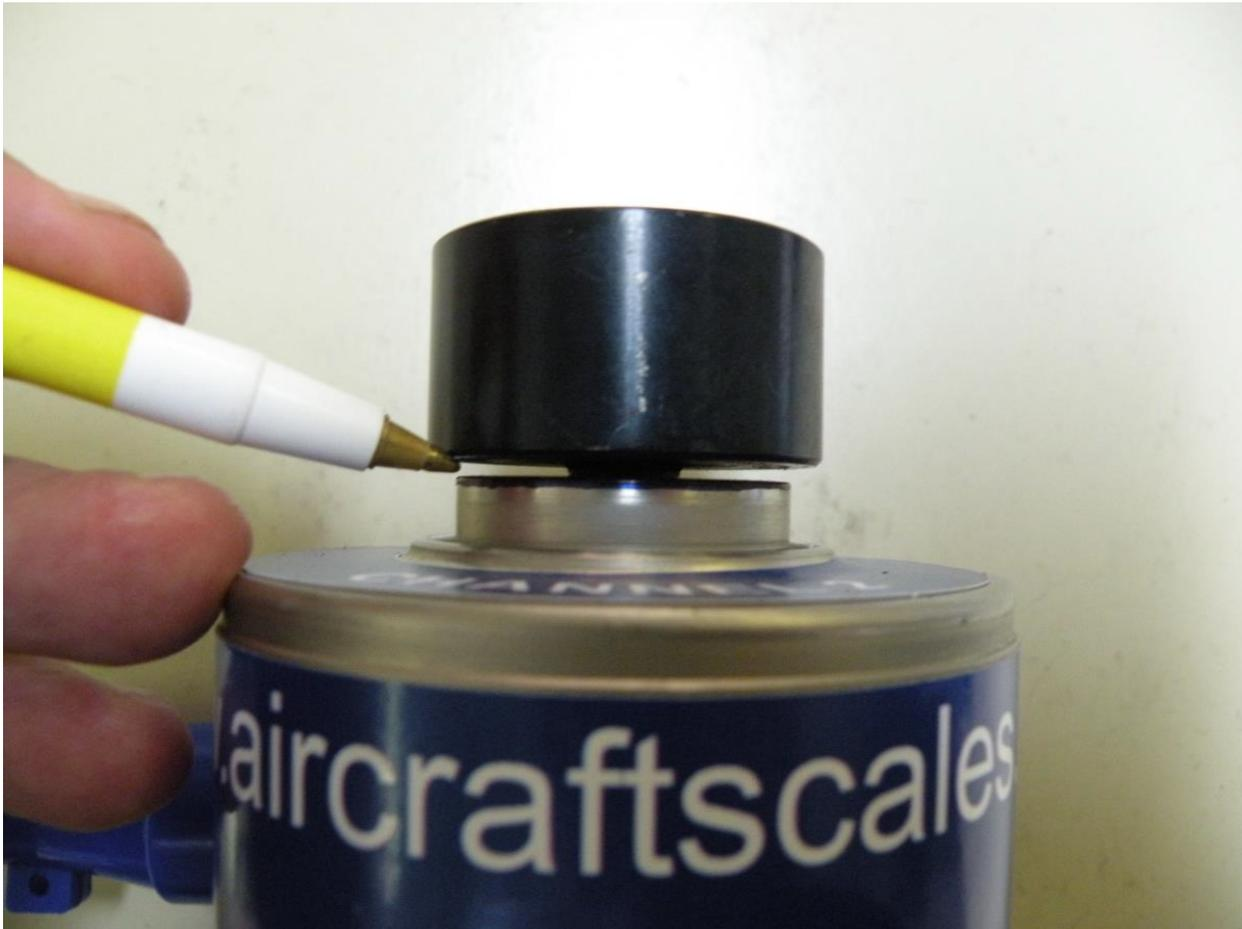
Below is a picture of an improper install, note that the adapter is not all the way bottomed and there is an air gap. Cells with air gap will read incorrectly, can be damaged and may cause damage to the aircraft.
