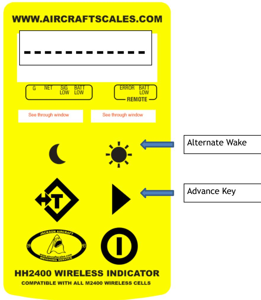
Use the Advance key to advance the indicator to the input cell not awake. Once there, hold down and release the Alternate wake key while 2ft to 4ft away and pointing the indicator at the cell in the horizontal position. The cell will wake
