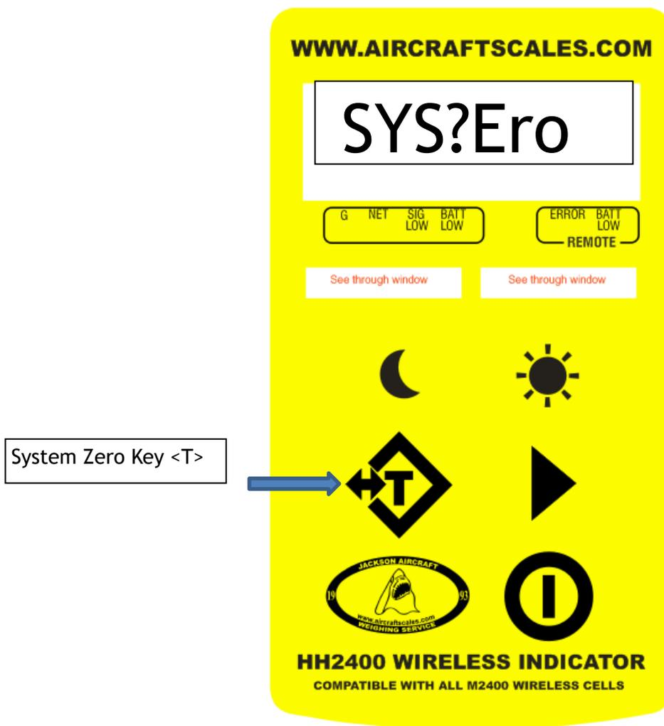
On power up the unit is set to default and read the total weight of all cells. In this mode, pressing the tare key and holding it will force a System Zero.
