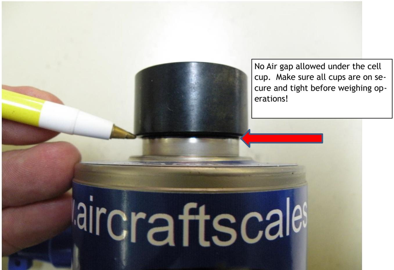
Note: It is very important that the cell top jack pad adapters are screwed in all the way as shown with no air gap, adapter must bottom on the cell top.
