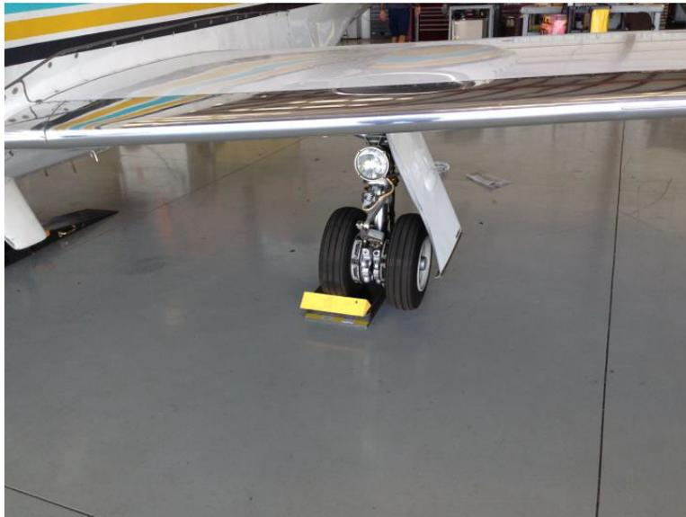
Note: Center the wheel directly on the center of the platform.
